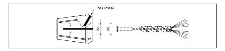
In this type of collets, slots are SEALED with rubber so that collets can be used for coolant through application and can withstand coolant pressure upto 1500 psi (110 bar)
