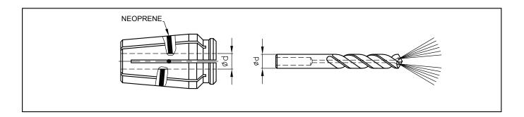
In this type of collets, slots are SEALED with rubber so that collets can be used for coolant through application and can withstand coolant pressure upto 1500 psi (110 bar)
